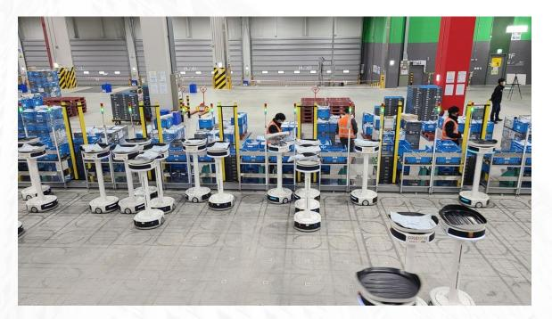
These AGVs save human workers from the back-breaking labor of moving hundreds of thousands of packages each day, reducing manual workloads by nearly 65%. And the autonomous factory has delivered a major boost for Coupang's bottom line.
