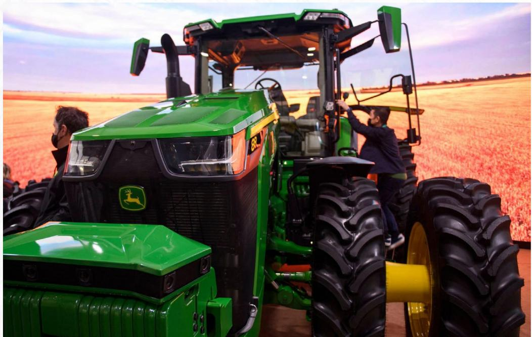
The 8R comes with 12 360-degree cameras that feed images into a neural network, a form of AI software modeled after the human brain. In approximately 100 milliseconds, the 8R's neural network classifies each image pixel from its cameras, allowing the tractor to make instantaneous decisions about whether it should stop, keep moving, or change directions. The system is linked to a live GPS feed, which farmers can monitor from the Deere Operations Center.
